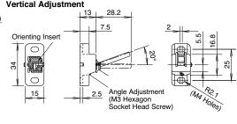
The orientation of actuator adjustment (horizontal/vertical) can be changed using the orienting insert (white plastic) installed on the back of the actuator.
