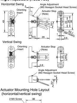
Note: The actuator stop is supplied with the actuator and used when adjusting the actuator position. Remove the actuator stop after the actuator position is determined.
