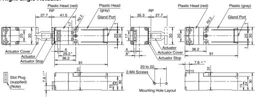
Note: Plug the unused actuator insertion slot using the slot plug supplied with the safety interlock switch.
